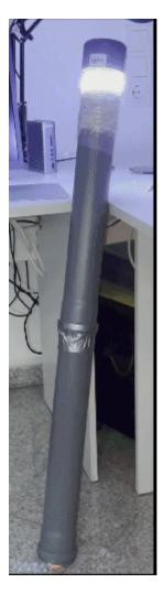
The input device is currently only one single push button<sup>2)</sup>. The use of this button is reported to the commander by two subsequent events. First when it is pushed down and second when it is released.
